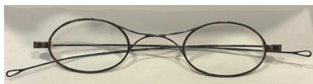
Figure 3. Steel X-bridge pair of spectacles from the estate of Margaret Fristoe Beckwith, measured at +3.50 diopters.
